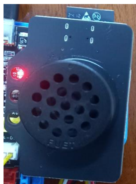
Figure 9: Activate speaker warning, LED turns red
